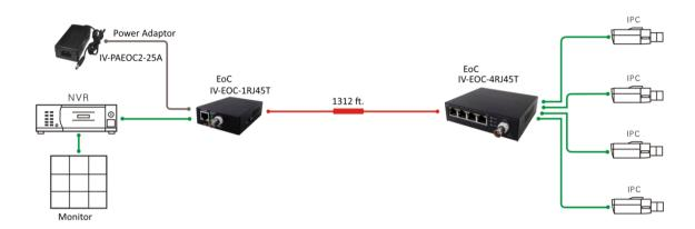
7 Local side: IV-EOC-1RJ45T with DC56V 2A power adaptor to POE remote side and camera Remote side: distance to 1640 ft. apply a IV-EOC-4RJ45T and three camera powered by local IPC 1.3 million pixels 720P, each 5Mbps Stream
