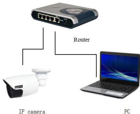
Picture 5 Network structure
