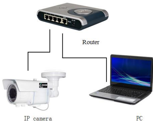
Picture 5 Network structure
